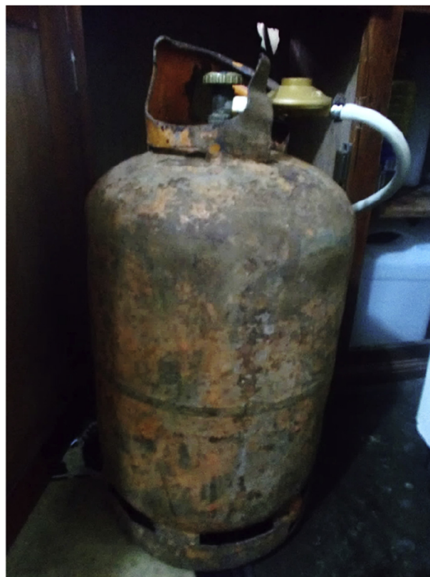
Fig. 10. Example of poor-quality LPG cylinder (P3, F, age 28, Peri-urban, Income 1).
