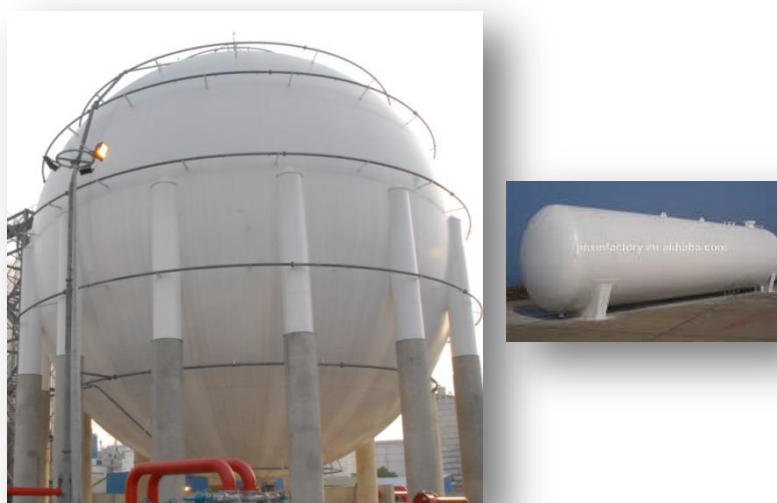
Figure 35. Examples of spherical and bullet LPG storage
